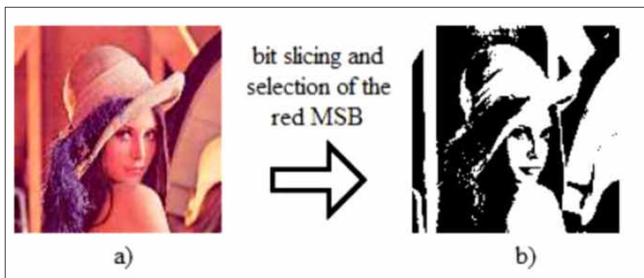
Figure 22. a) Lena's color image of 128-by-128-by-3-by-8 bits. b) Lena's MSB bitplane of the red channel with 128-by-128-by-1 bits.
